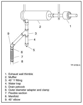
Figure 5-2 Exhaust System, Side Inlet Silencer
